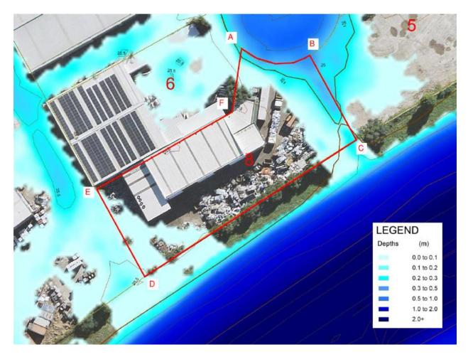
The Applicant has proposed mitigation measures to protect the water quality of the adjoining creek, ensure the development will not impede the natural recession of floodwaters in the area, and prevent material stored onsite from being washed offsite in significant flood events.
